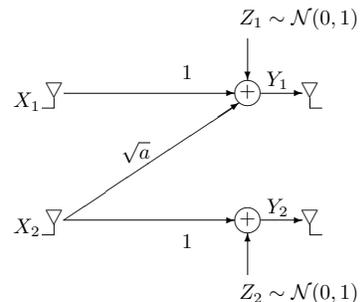
Fig. 1. A one-sided Gaussian interference channel in standard form.
