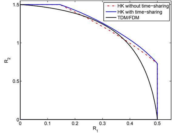
Fig. 3. The Han-Kobayashi achievable region with and without time-sharing for  $a = 0.5$ ,  $P_1 = 1$  and  $P_2 = 7$ . The TDM/FDM region is a subset of the HK scheme with time-sharing ( $\mathcal{R}_{\text{HK}}^{\mathcal{G}}$ ) in which in each subband only one user is allowed to transmit. It is seen that  $\mathcal{R}_{\text{HK}}^{\mathcal{G}}$  is strictly larger than the other two regions.
