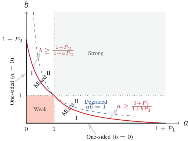
Fig. 4. Different classes of the interference channel defined by (1a)-(1b). We simplify the HK scheme for the one-sided interference regime as well as a large part of the mixed interference regime (labeled “Mixed II” in this figure). The figure is for  $P_1 = 4$  and  $P_2 = 2$ .
