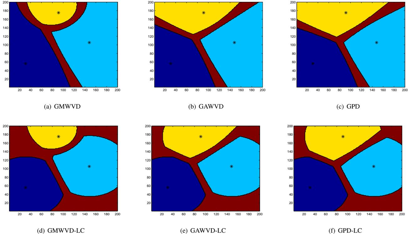
Fig. 1. Guaranteed diagrams for a field containing three sensors with different sensing radii and imperfect location information, for different algorithms. In Figs. 1(a)-1(c) the sensors' communication range is unlimited, while in Figs. 1(d)-1(f) it is limited. The regions in dark brown are the areas which are not assigned to any sensor, implying that a single-cell-based coverage hole detection is not applicable to them.
