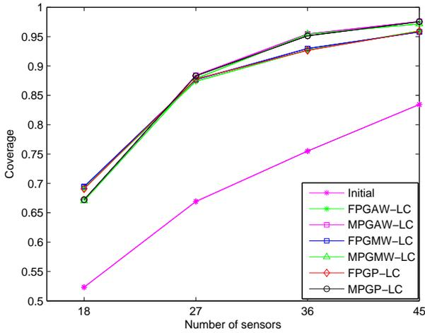
Fig. 3. Initial and final coverage versus the number of sensors for different algorithms. The FP- and MP-based algorithms make two separate clusters, and within each cluster there is not much difference between the final coverage.
