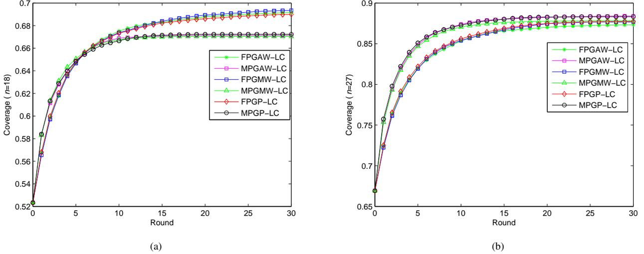
Fig. 2. Network coverage using different algorithms at various iterations: (a) for 18 sensors (b) for 27 sensors.
