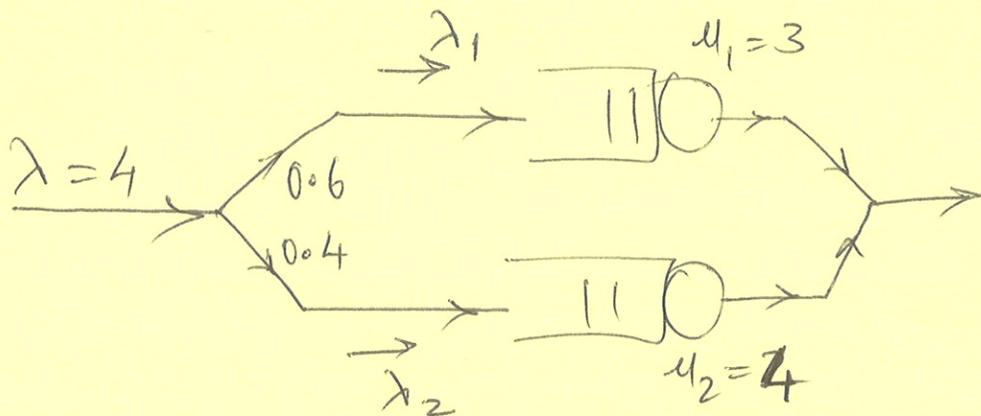
In the above diagram, of a standard  $M/M/1$  queues, the fractions  $0.4$  and  $0.6$  indicate the iid probabilities of routing arriving jobs to the two branches. Determine ~~the~~ the expected number of customers for the whole system. What is the expected response time for the whole system?
